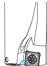
图4 内刃的钻头中心部附近的崩损 FIG. 4 Collapse near the center of the bit at the inner edge
